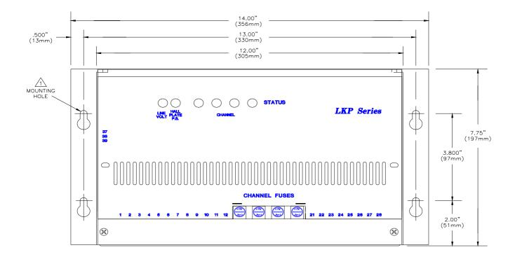
SECURE METER UNIT TO MOUNTING SURFACE WITH FASTENERS IN FOUR (4) LOCATIONS SHOWN. KEYHOLES IN MOUNTING PLATE WILL ACCOMODATE EITHER #10(5mm) SCREW OR 1/4"(6mm) SCREW OR BOLT.
